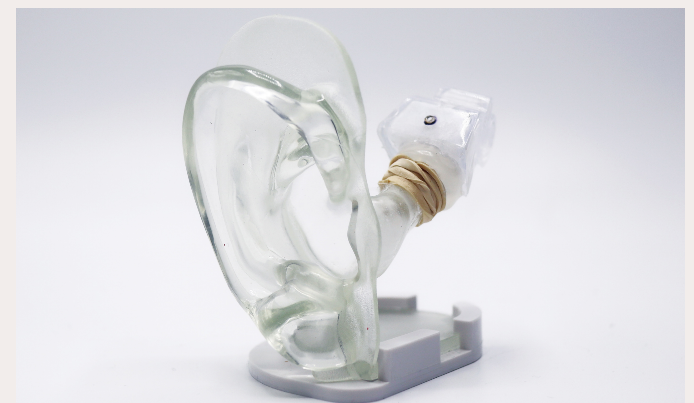
To develop our algorithm in controlled circumstances, we modified earbuds and plastic model ears to collect data.
