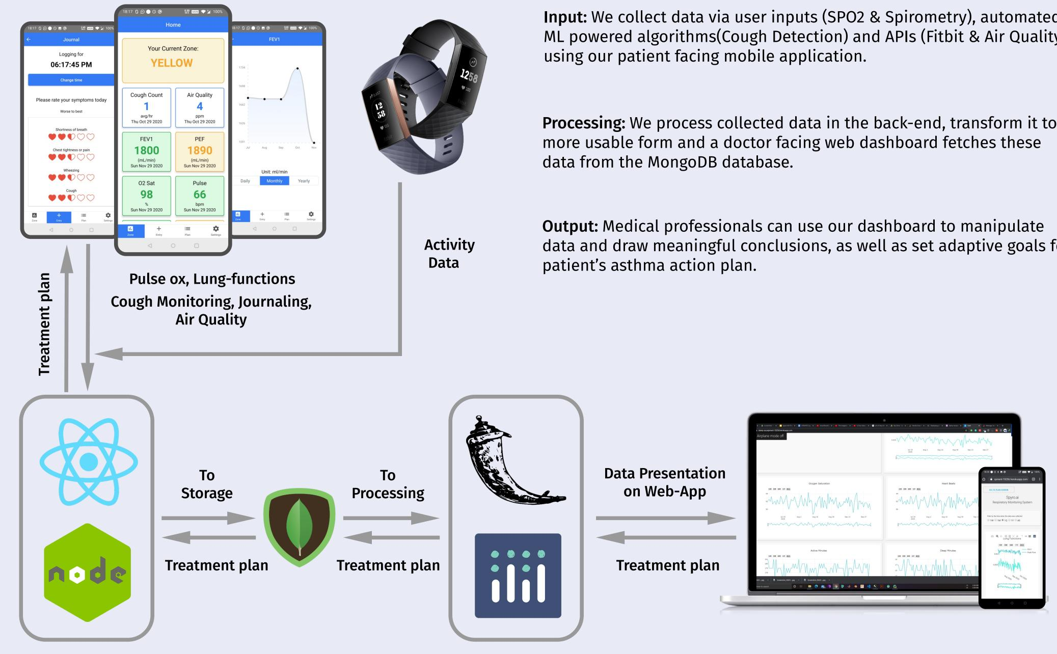
**Input:** We collect data via user inputs (SPO2 & Spirometry), automated ML powered algorithms(Cough Detection) and APIs (Fitbit & Air Quality)
