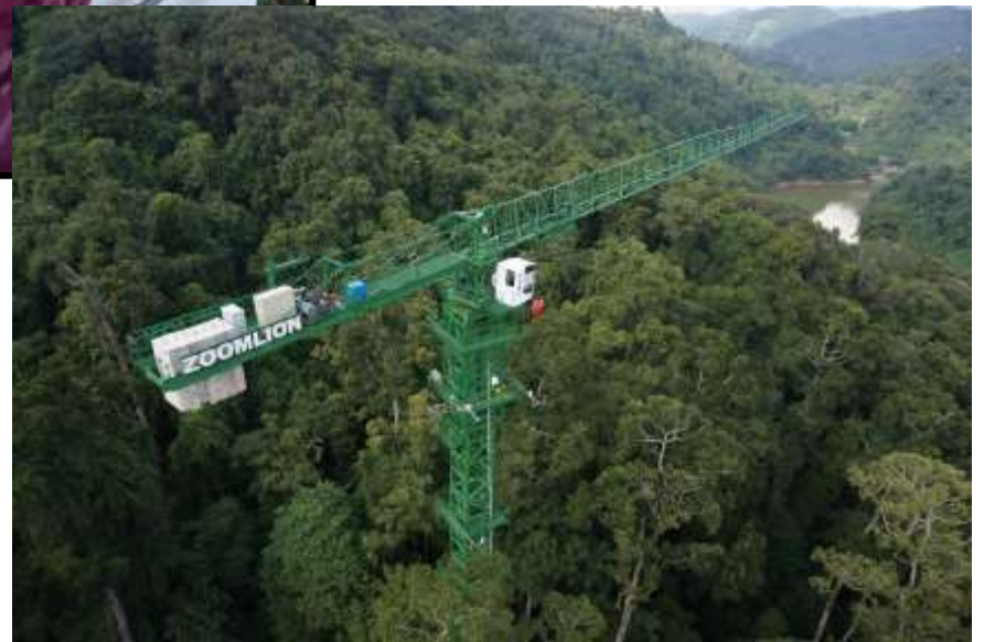
Canopy crane (80 m high, 60 m jib)
