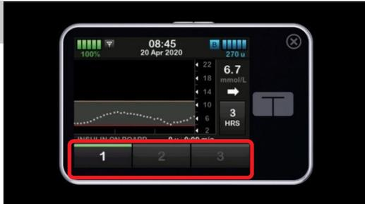
On the screen tap **1-2-3** in sequence to unlock the pump. The pump home screen will be displayed.
