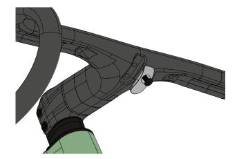
Release the bolt and remove the cover.
