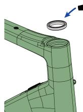
Lightly grease the upper headset bearing and then install in upper headset cup.
