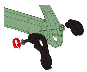
Apply Loctite 243 on bolt threads. Thread the bolt in but do not tighten, this will allow the insert to align when installing the axle
