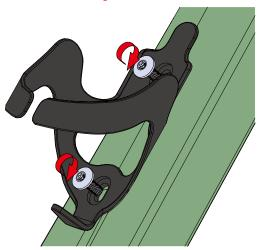
Install cages and tighten M5 bolts with T20 Torx to 2 Nm.
