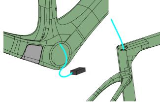
Route the Di2 seat post cable from seat tube to the bottom bracket (internal port). Connect to the Shimano Di2 Junction B according to Shimano's instructions.
