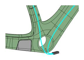
Route the downtube Di2 cable through slot in the headtube.
