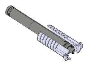
Place the battery holders around the Di2 battery. The male shell grooves must match with the female battery groove.
