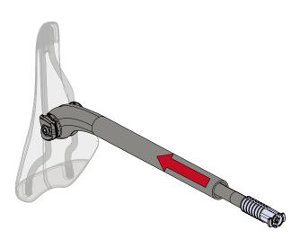
1-6 Before assembly, the wedge must be adjusted so that both bolts are flush with the outer surface of the wedge (red line of the picture). Keep in mind that the M4 bolt only holds the wedge pieces together and plays no part in tightening the seat post.
