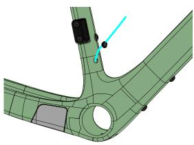
Torque the barstem to **5.2Nm**
