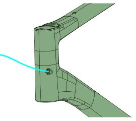
Exit the hyduaulic hose through slot in the headtube
