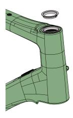
Lightly grease and install compression ring.
