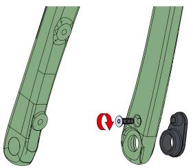
Apply Loctite 243 on bolt threads. Thread the bolt in but do not tighten, this will allow the insert to align when installing the axle
