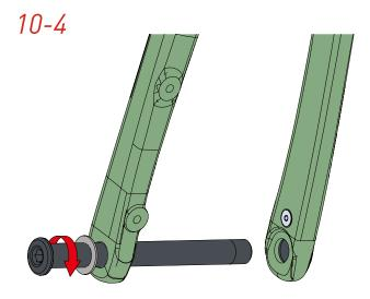
Remove the thru-axle and remove the hub. Install front wheel and tighten the thru axle (with the nylon washer) to **12Nm.**
