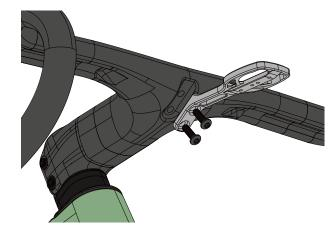
Install the computer mount and tighten the 2 bolts to **2 Nm.**
