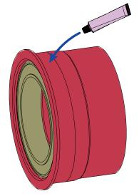
Apply Loctite 641 on the grooves of the both bottom bracket cups.
