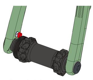
After ensuring the dropout insert is correctly aligned, tighten the dropout bolt to **1 Nm.**
