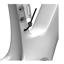
Route the front derailleur Di2 cable through the seat tube hole to the bottom bracket exit port.
