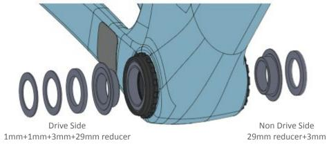
For Shimano Hollowtech II cranksets, install the included 24mm Wheels MFG reducers and spacer in the following sequence.
