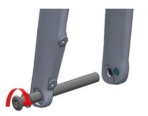
front wheel and tighten the thru axle (with the nylon washer) to **12Nm.**
