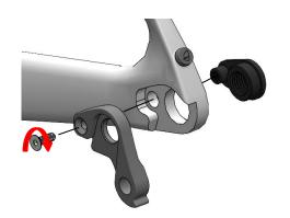
Apply Loctite 243 on bolt threads. Thread the bolt in but do not tighten, this will allow the insert to align when installing the axle
