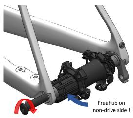
Install a rear hub in the dropout with the free hub on non-drive side. This will allow better access for the next step. Install the thru-axle with the nylon washer and tig hten to **12Nm.**
