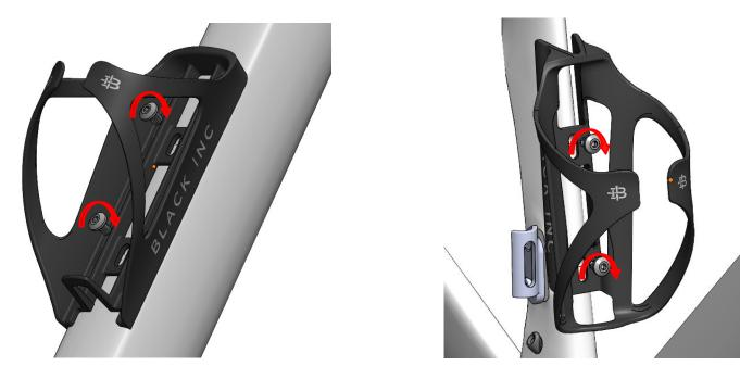
Install cages and tighten M5 bolts with Hex3 to 2 Nm.
