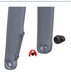
Apply Locate 245 on port arreaus. Threau the bolt in but do not tighten, this will allow the insert to align when installing the axle Install a front hub in the dropout with the free hub on non-drive side. This will allow better access for the next step. Install the thru-axle with the nylon washer and tighten to **12Nm**
