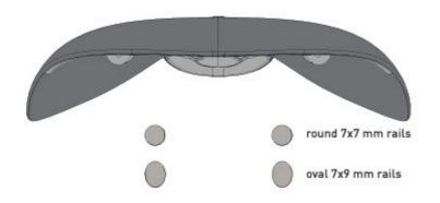
Factor frame sets are shipped with 7X9 mm outer rail clamps for carbon rail saddles. 7x7 mm outer rail clamps for traditional saddle rails are available through your Factor dealer.
