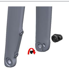
Apply Loctite 243 on bolt threads. Thread the bolt in but do not tighten, this will allow the insert to align when installing the axle Install a front hub in the dropout with the free hub on non-drive side. This will allow better access for the next step. Install the thru-axle with the nylon washer and tighten to **12Nm**
