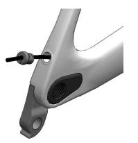
Route the rear derailleur Di2 cable through the chainstay.
