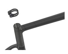
Grease the area between the Clamp and the frame with a dielectric grease to prevent corrosion
