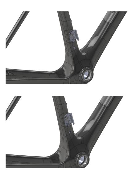
If you are using a 1x setup, remove the FDM and set aside. Install the provided blanking plates for the FD mounting holes. Note you may benefit from a small dab of adhesive or silicone when installing these as they can rattle out with time.
