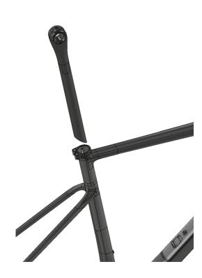
Apply frame assembly compound to the 27.2mm round post
