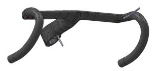
Snake hoses through the bar, respecting which is left and which is right and corresponding front/rear brakes
