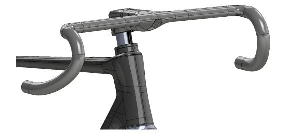
Gently pull the hoses through the bar while starting to locate it over the steerer tube.
