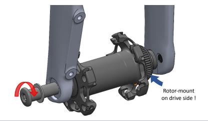
After ensuring the dropout insert is correctly aligned, tighten the dropout bolt to **1 Nm**.
