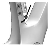
Route the front derailleur Di2 cable through the seat tube hole to the bottom bracket exit port.
