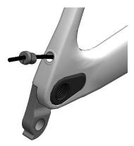
Route the rear derailleur Di2 cable through the chainstay.
