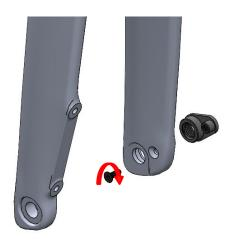
Apply Loctite 243 on bolt threads. Thread the bolt in but do not tighten, this will allow the insert to align when installing the axle
