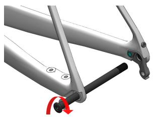
Remove the thru-axle and remove the hub. Install the rear wheel and tighten the thru-axle (with the nylon washer) to **12Nm**.
