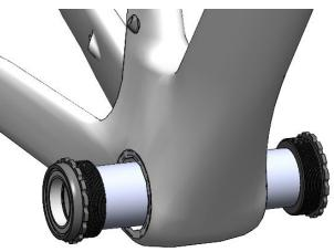
Thread the cups into the frame and torque the cups down to 30nm for the drive side and 40nm for the non drive side. We recommend using Park Tool BBT-47.
