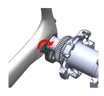
After ensuring the dropout insert is correctly aligned, tighten the dropout bolt to **1 Nm**.
