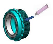
Apply a layer of good quality assembly paste to the threads of both bottom bracket cups. We recommend assembly paste from Morgan Blue (Aquaproof Paste) or r.s.p. (Creak Freak Assembling Paste).
