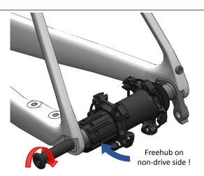
Install a rear hub in the dropout with the free hub on non-drive side. This will allow better access for the next step. Install the thru-axle with the nylon washer and tig hten to **12Nm.**
