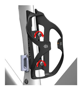
Install cages and tighten M5 bolts with Hex3 to 2 Nm.
