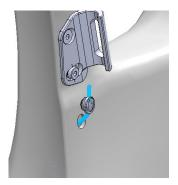
Route the front derailleur Di2 cable through the seat tube hole to the bottom bracket exit port.
