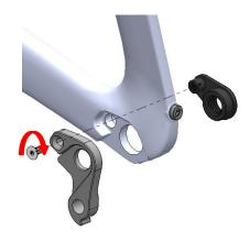
Apply Loctite 243 on bolt threads. Thread the bolt in but do not tighten, this will allow the insert to align when installing the axle
