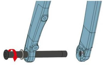
Remove the thru-axle and remove the hub. Install front wheel and tighten the thru axle (with the nylon washer) to **12Nm.**
