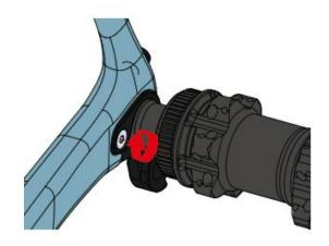
After ensuring the dropout insert is correctly aligned, tighten the dropout bolt to **1 Nm.**
