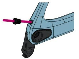
Route the rear derailleur Di2 cable through the chainstay.
