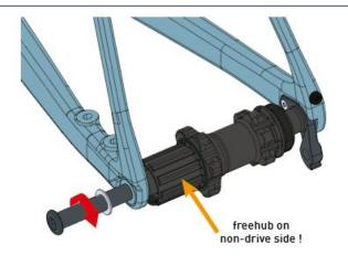
Install a rear hub in the dropout with the free hub on non-drive side. This will allow better access for the next step. Install the thru-axle with the nylon washer and tig hten to **12Nm**.
