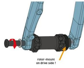
After ensuring the dropout insert is correctly aligned, tighten the dropout bolt to **1 Nm.**
