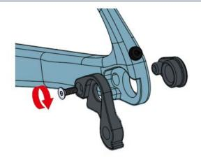
Apply Loctite 243 on bolt threads. Thread the bolt in but do not tighten, this will allow the insert to align when installing the axle
