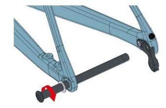
Remove the thru-axle and remove the hub. Install the rear wheel and tighten the thru-axle (with the nylon washer) to **12Nm.**
