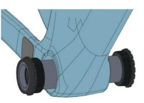
Thread the cups into the frame and torque the cups down to 30nm for the drive side and 40nm for the non drive side. We recommend using Park Tool BBT-47.
