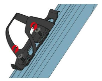
Install cages and tighten M5 bolts with T20 Torx to 2 Nm.
