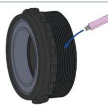
Apply a layer of good quality assembly paste to the threads of both bottom bracket cups. We recommend assembly paste from Morgan Blue (Auqaproof Paste) or r.s.p. (Creak Freak Assembling Paste).
