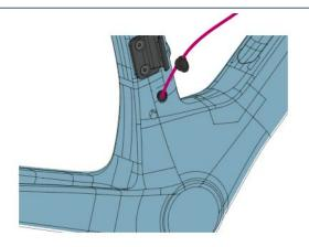
Route the front derailleur Di2 cable through the seat tube hole to the bottom bracket exit port.
