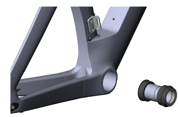
Clean the inside of the frame bottom bracket & the bottom bracket cups with an isopropyl alcohol.
