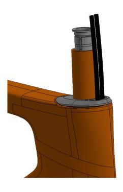
Apply carbon assembly paste to the compression plug, install in steerer, and tighten to 8Nm
