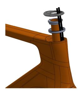
Grease and install the upper bearing, Split ring, and dust cap. Make sure the hoses go through the appropriate openings on the split ring and dust cover.
