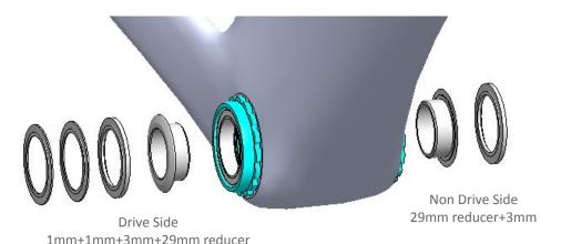
For Shimano Hollowtech II cranksets, install the included 24mm Wheels MFG reducers and spacer in the following sequence.
