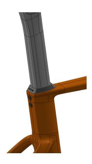
Install the SP into the frame. Tighten the grub screws using a high quality allen key to 4Nm, alternating between the bolts to bring the assembly up to tightness in a uniform fashion. Failure to alternate torque may result in frame or seat post cracking and void the warranty.
