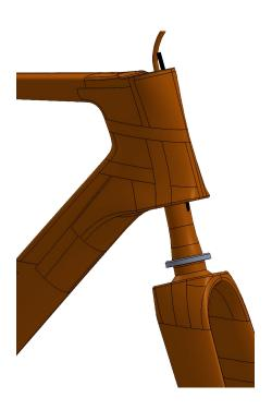
Pull the hose through the lower bearing, grease the lower bearing seat, and install the fork and bearing into the frame
