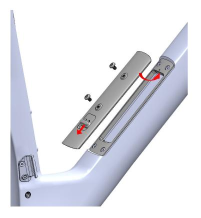
Insure that the factory installed bezel bolts are tightened (2Nm). Install cover and tighten M5 WB bolts with a high quality 3mm Hex head to **2 Nm**.
