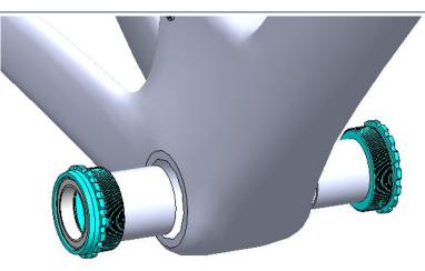
Thread the cups into the frame and torque the cups down to 30nm for the drive side and 40nm for the non drive side. We recommend using Park Tool BBT-47.
