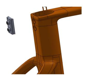
Apply a thick coat dielectric grease, or frame prep compound to the rear of the SP clamp assembly
