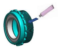
Apply a layer of good quality assembly paste to the threads of both bottom bracket cups. We recommend assembly paste from Morgan Blue (Aquaproof Paste) or r.s.p. (Creak Freak Assembling Paste).
