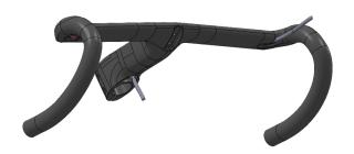
Snake hoses through the bar, respecting which is left and which is right and corresponding front/rear brakes
