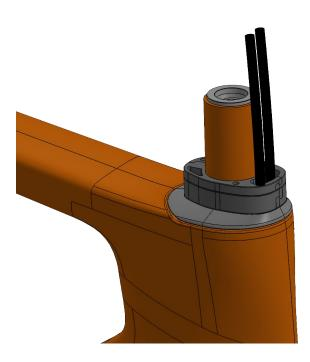
Install the relevant number of spacers. Note max spacer stack not to exceed 4cm
