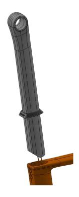
Install the SP gasket around the post. Once the gasket is on (not before) apply a generous coating of carbon assembly compound to the seat post.
