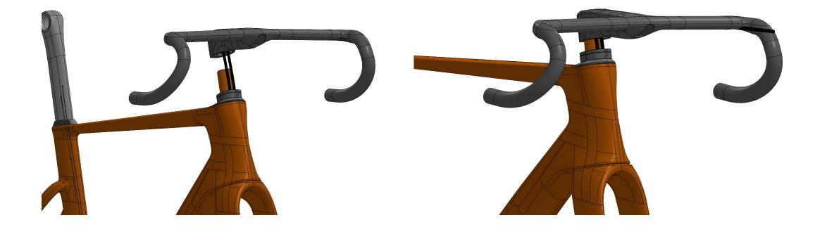
Gently pull the hoses through the bar while starting to locate it over the steerer tube.
