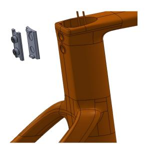
Grease the area between the two plates to prevent corrosion
