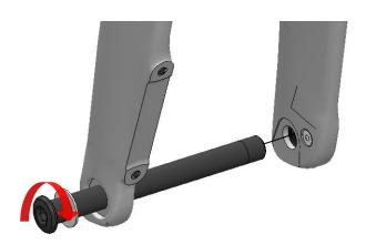
Remove the thru-axle and remove the hub. Install front wheel and tighten the thru axle (with the nylon washer) to **12Nm.**
