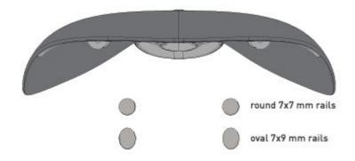
Factor frame sets are shipped with 7X9 mm outer rail clamps for carbon rail saddles. 7x7 mm outer rail clamps for traditional saddle rails are available through your Factor dealer.
