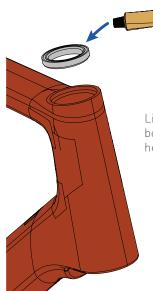
Lightly grease the upper headset bearing and then install in upper headset cup.
