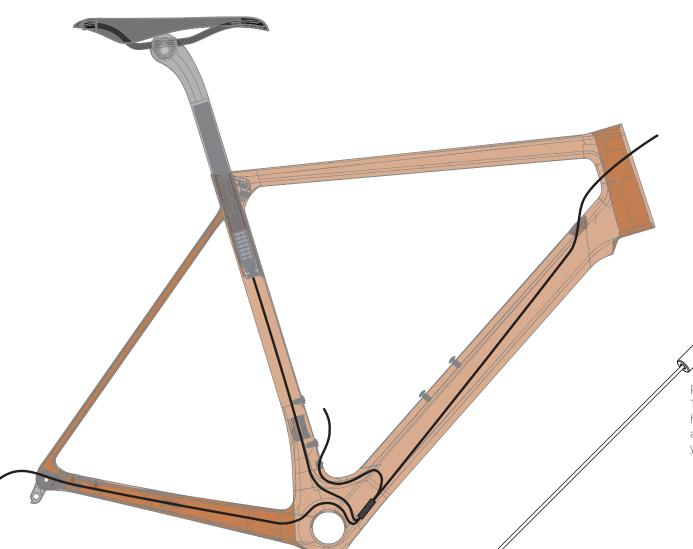
Park Tool offers an excellent internal cable routing kit (Park Tool IR-1) to help you easily route your cables. If you do not have access to this kit you can use a derailleur inner wire and a 5mm metal cable ferrule to route your wires.
