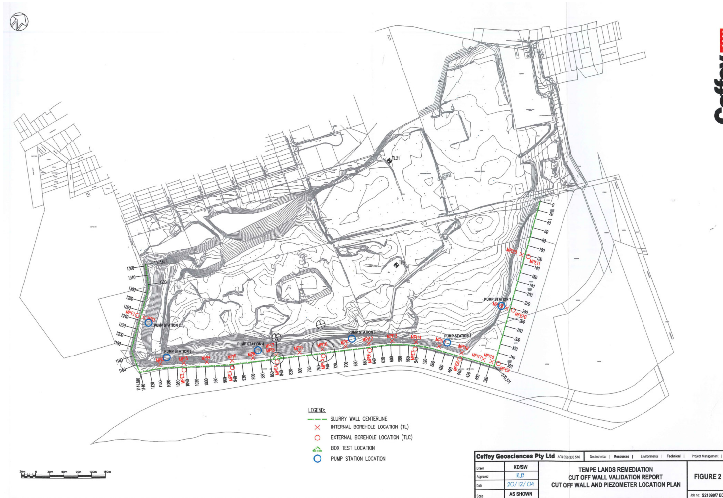
Figure 5-1: Monitoring wells and leachate pump pits located along the bentonite wall
