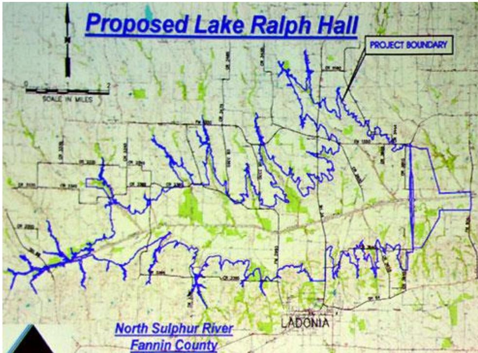
The reservoir is part of long-range plans to meet the water needs of the burgeoning population in North Texas, while also resolving an erosion problem of epic proportions. In order to mitigate flood damage along North Sulphur River, in 1928-29 a 16-foot wide, 10-foot deep channel was dug to parallel the river. That channel is now more than 300-foot wide and 60 feet deep, 10 times its original size, and growing.
