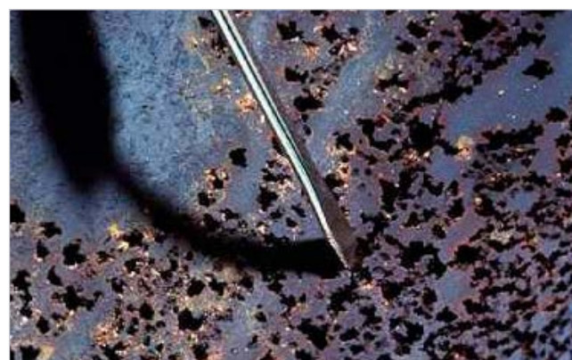
Figure 3 – Pitting corrosion by an aggressive medium (www.watertechnologies.com - December 2023)
