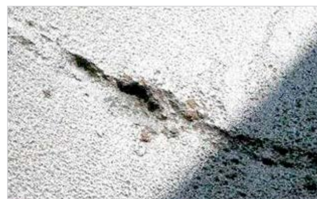
Figure 4 – Metal loss in a girth weld (NDTG 2007)
