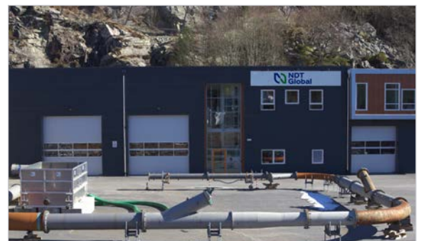
Pump trial setup including diameter change and wye passage.
