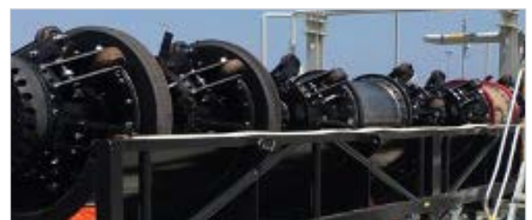
ART Scan tool at receiver after 900 km (~600 miles) inspection.
