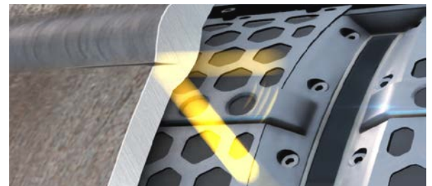
Direct sizing capabilities using the crack tip
