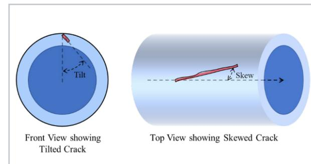
Figure 2 – Schematic of tilted and skewed ideal cracks.
