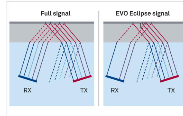
Figure 3 – The Pitch and Catch technology principle. Full signal with no shading (left) and eclipsed signal due to a feature (right). The CW Sensor (Sensor 1) is in receiving mode while the CCW (Sensor 2) is in transmitting mode.
