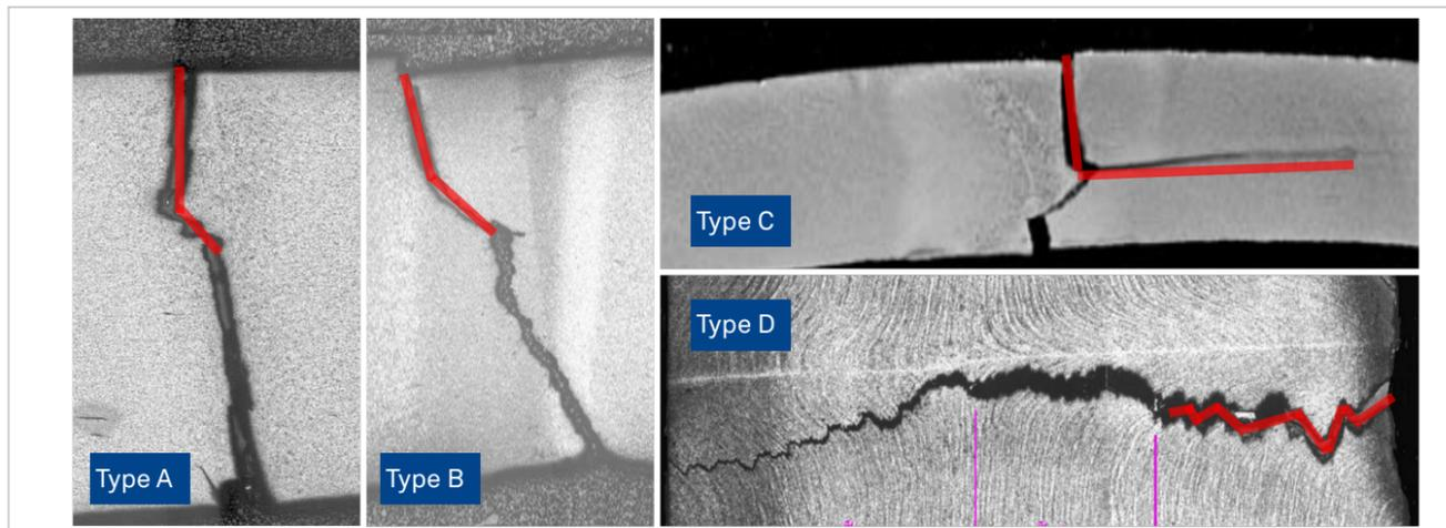
Figure 5 – Sample of hook crack morphologies. Red lines indicate the fundamental crack morphology (Hartl, K. et al. 2021).
