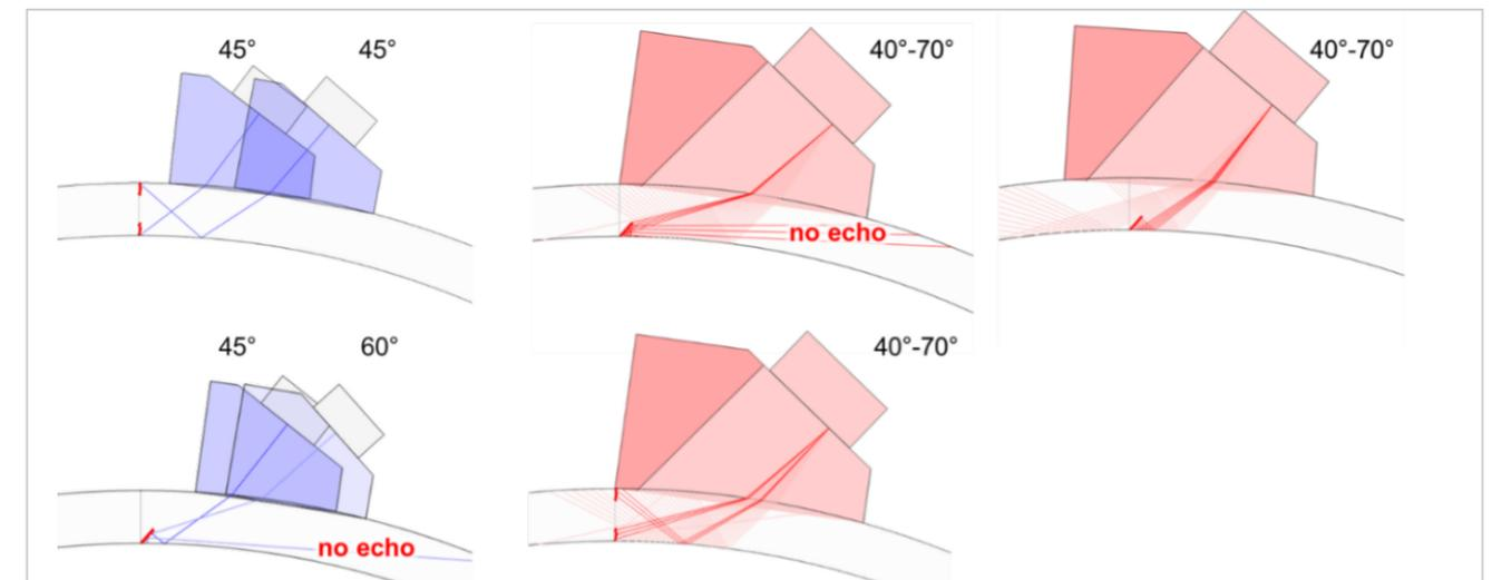
Figure 4 – Sound paths for SWUT (blue) and PAUT (red) for tilted cracks (top) and radial, surface-connected cracks (bottom). Note, that the tilted reflector may be missed depending on the probe's angle (for SWUT) and position (for PAUT sectorial scans), as the reflections are guided away from the probe.
