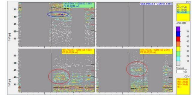
Figure 7 – B-Scan data for a verified hook crack. Upper scans correspond to CW sensors and bottom scans to CCW sensors.
