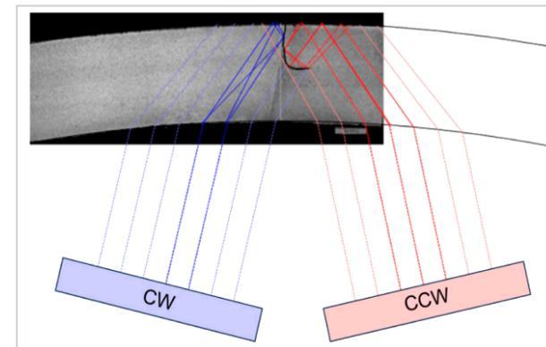
Figure 6 – Scheme of a hook crack detected by clockwise and counterclockwise sensors. Colour lines simulate the sound beam, and the stronger ones indicate reflections from the flaw back to the sensors.
