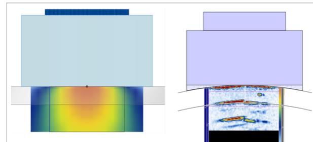
Figure 10 – Left: TFM sensitivity map for the setup using a LL-mode (but neglecting the pipe curvature). Right: Sketch of probe above the seam weld and the corresponding T-scan for a laminar reflector clockwise from the centerline.
