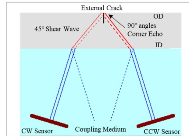
Figure 1 – Schematic of clockwise and counterclockwise UT sensors interacting with an ideal crack. The CW Sensor is transmitting while the CCW Sensor is also in transmission mode (no Pitch and Catch technique).
