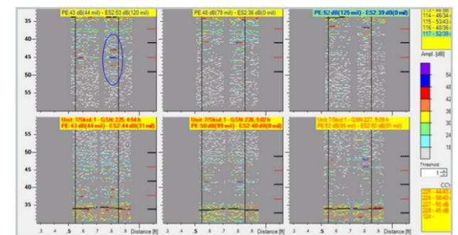
Figure 8 – B-Scan data for a verified hook crack.
