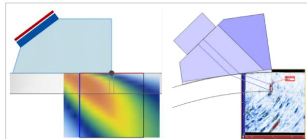
Figure 9 – Left: TFM sensitivity map for the setup using a TT-mode (but neglecting the pipe curvature). Right: Sketch of the probe in 90° skew position and the corresponding T-scan for an internal reflector on the weld centerline. Additional echoes originate from small impurities within the steel.
