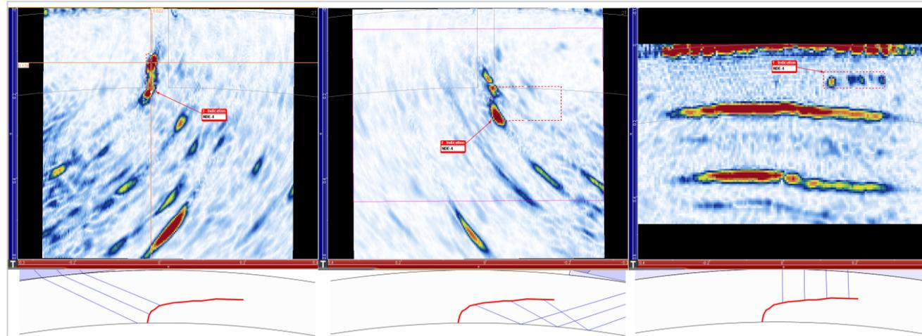
Figure 11 – TFM T-scan images of a hook crack. From left to right: probe shooting clockwise (TT-mode, 90° skew), counterclockwise (TT-mode, 270° skew), and vertical (LL-mode). The sketches below indicate the main direction of the ultrasonic signals.
