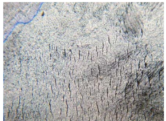
Circumferential crack field detected with ILI results using UCc
