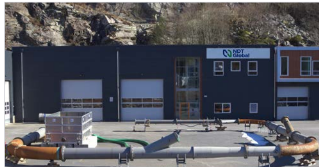
Figure 11 – Pump Trial Setup including diameter change and Wye passage
