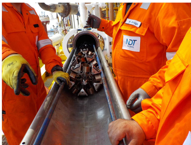
Figure 5. Ump sensor carrier during the loading procedure.
