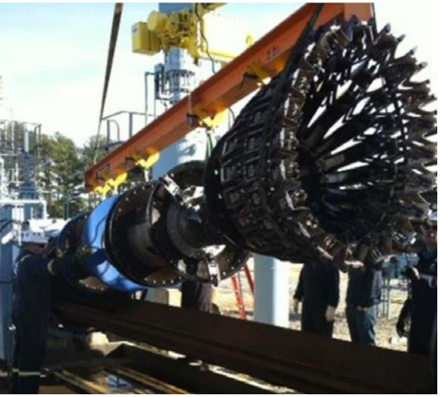
Figure 3 – NDT Global UC tool in launcher with tray configuration
