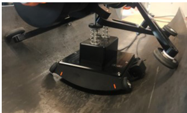
Figure 4. ETEC internal crack detection prototype tool.
