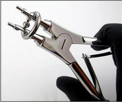
**Figure 28.** Ring expanding pliers being used to expand ring.
