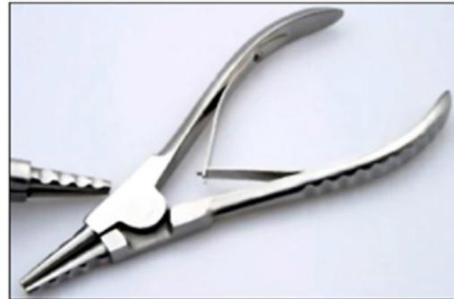
**Figure 27.** Ring expanding pliers.
