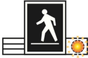
Pedestrian activated crosswalk — prepare to stop if the light is flashing
