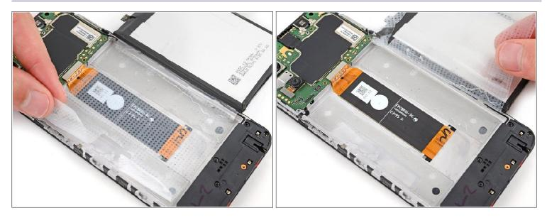
• Use your fingers to peel the battery's plastic film from the frame.
