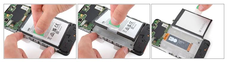
• With one hand, fold the clear outer tabs out of the way of the battery and firmly hold them down to secure the frame.
