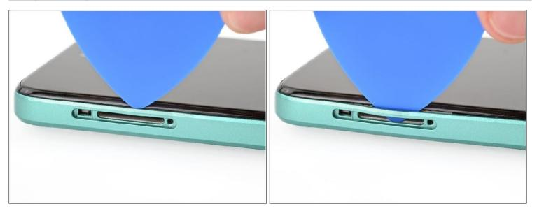
Insert the tip of an opening pick between the back cover and frame, at the SIM card tray cutout.
