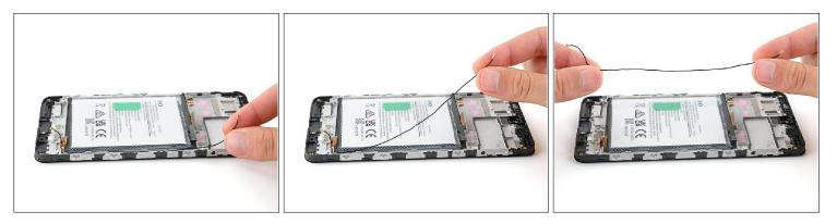
• Use your fingers to lift the black antenna cable out of its groove on the right edge of your phone.
