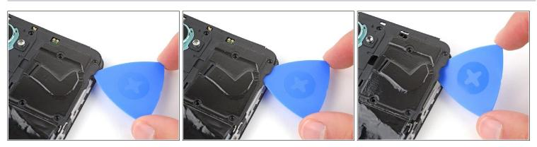
• Insert an opening pick between the right edge of the motherboard cover and
