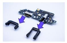
• Remove the rubber parts from the charging port
