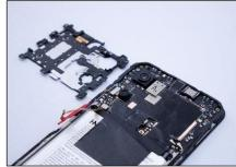
• Insert the opening tool under the right edge of the motherboard cover and carefully lift it
