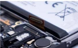
• Disconnect the main flex cable from the charging port circuit, use Spudger or opening stick
