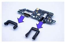
• Remove the rubber parts from the charging port
