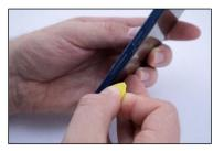
• Continue sliding the opening tool along the bottom side
