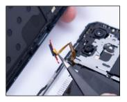
• Take a note of the actual location and position of fingerprint reader cable for later assembly
