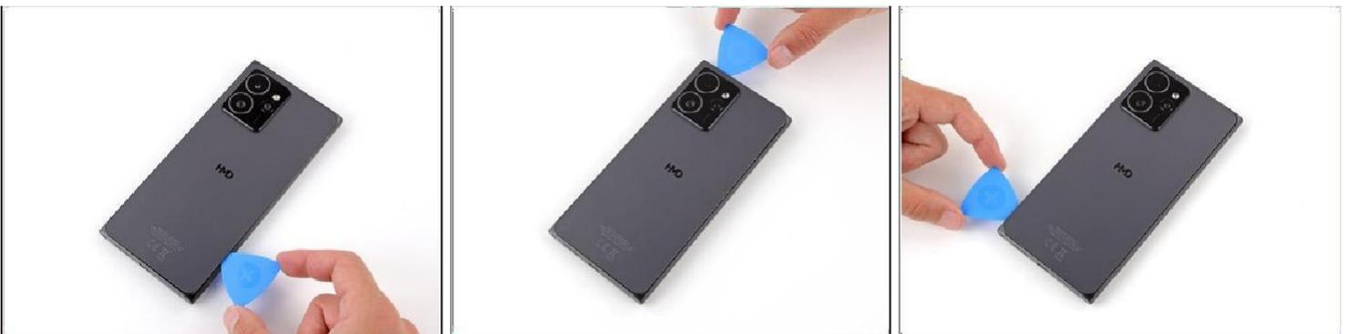
● Continue sliding the pick under the perimeter of the back cover to fully separate
