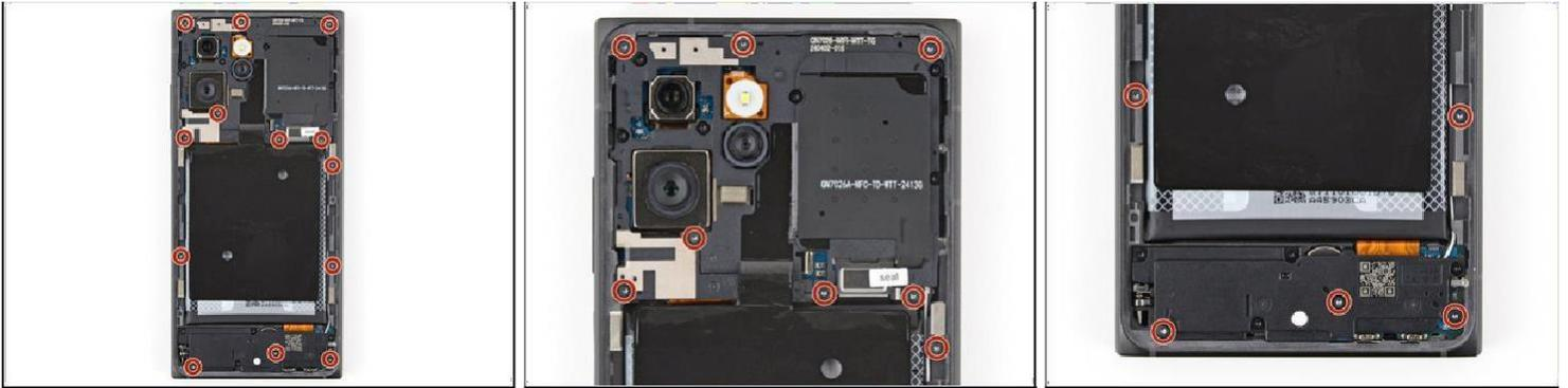
Use a T3 Torx screwdriver to remove the thirteen 4.9 mm-long screws securing the screen to the frame.
