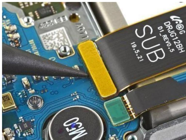
connector and pry up to disconnect it.
