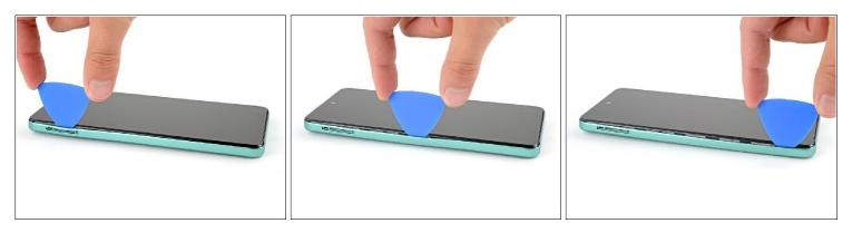
• Position the opening pick straight down and slide it along the left edge to begin unclipping the back cover.
