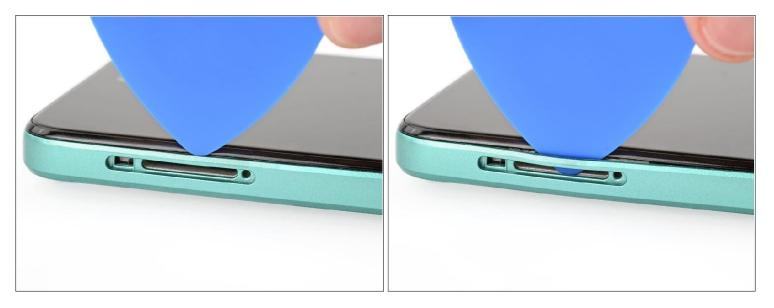
• Insert the tip of an opening pick between the back cover and frame, at the SIM cardtray cutout.
