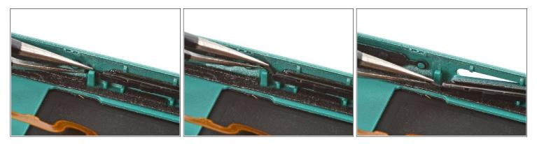
(i) If your replacement back cover doesn't come with a power button pre-installed, follow the next two steps to remove and transfer it.
