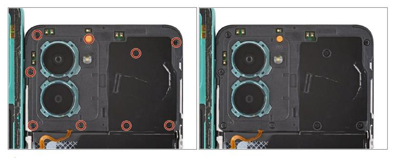
$\triangle$  Be very careful not to puncture the battery with your Cross-head screwdriver.
