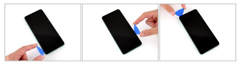
• Continue sliding the pick around the perimeter of your phone until the back cover is fully unclipped.
