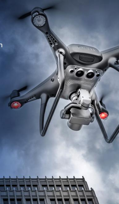
**Multipath effects:** Can the UAV recognise and correct for 'multipath' effects caused by the GNSS signal bouncing off tall buildings?
