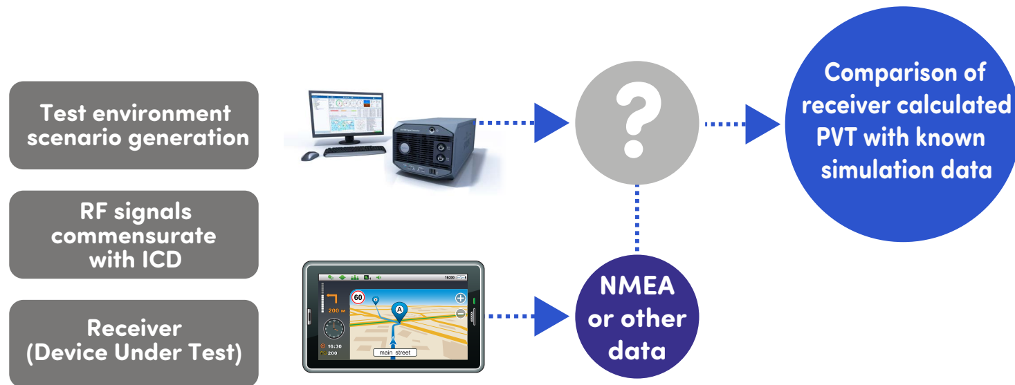
Figure 2. Simulation test set-up.
