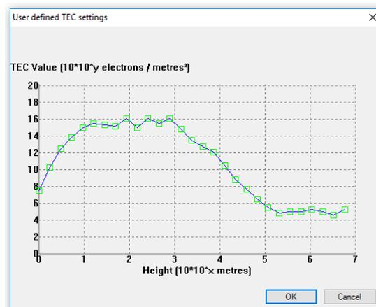
It is possible to perform a phased transition from the Terrestrial to the TEC model at a user-defined altitude for a simulated spacecraft launch or re-entry trajectory that is provided in a file or via remote control.
