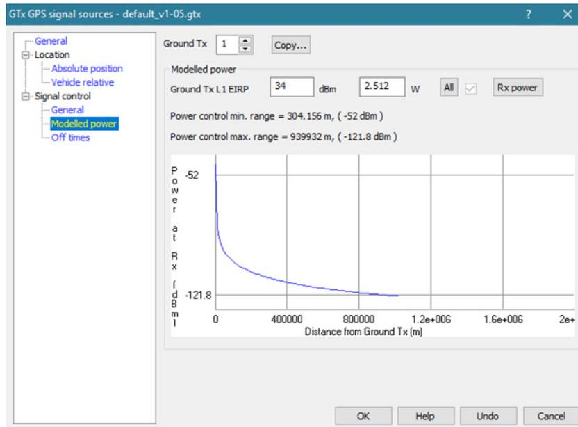
Figure 22 Power vs distance modelling for GTx
