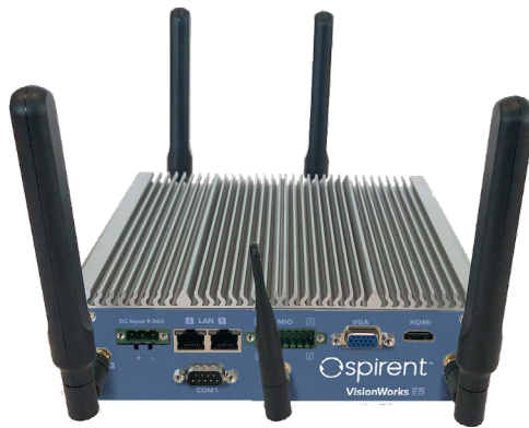
The VisionWorks E5 is a rugged test platform for deployment in indoor or outdoor locations
