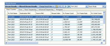
HyperFilters segregate each stream into different MAC addresses, IP addresses, ToS levels or any other user-defined characteristics of the received traffic.
