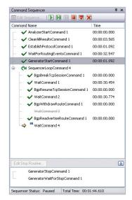
Users can create detailed and automated control over test events using the command sequencer.
