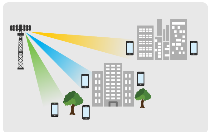
Figure 8. MIMO beams are used in reflection rich environments
