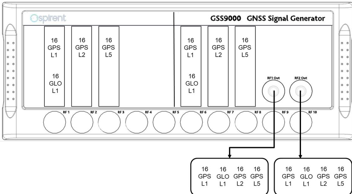
**Figure 6 Example of a dual-RF Output, 6-bank system**
