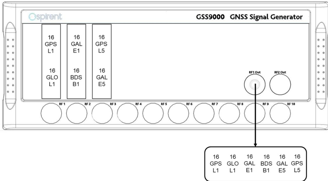
**Figure 5 Example of a single output, 3-bank system**
