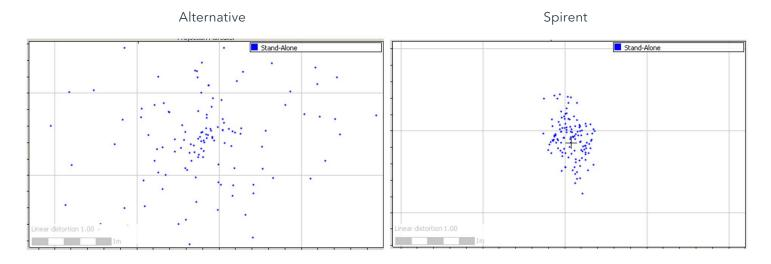
Due to a phase noise issue, the low quality simulator introduced inaccuracies of several metres.
