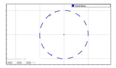
With the Spirent simulator, the receiver produced an accurate circle. But with the alternate test set simulating the signals, the receiver failed to achieve satellite lock at all. Again, under development conditions, this second result could be interpreted as a serious fault in the device under test, when in fact the issue is with the simulator itself.
