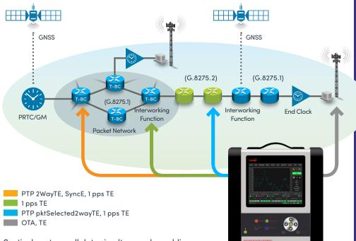
Sentinel captures all data simultaneously enabling you to correlate timing performance at different points in the network, even between different timing architectures.
