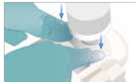
4. Press connector base onto your Ultrawave XS device.
