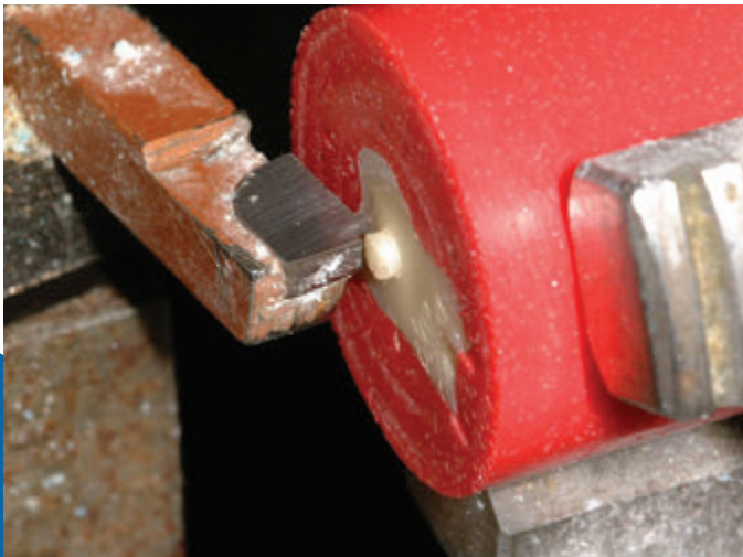
Dentin milled away leaving a protrusion for shear strength testing.
