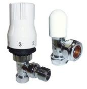
Warrior TRV's are self regulating valves fitted to radiators in a hot water based central heating system to control the temperature of individual rooms by changing the flow of hot water to the radiator.
