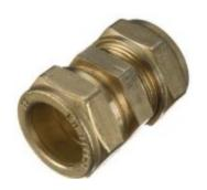
Compression fittings are designed to mechanically create a joint between the fitting and the pipe. When tightening the nut, you are compressing the olive onto the tube, creating a permanent seal.
