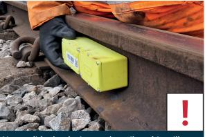
Never slide the device on the rail as this will damage the switch. If the position is not the one you want, remove and re-install it.
