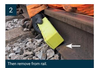
Data transmission (deployment) of the device will start after connection to the rail and will end at the point of device removal.
