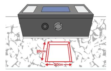
6. Once the unit has been secured to rail, remove an area of approx 20cm x 20cm in the ballast below the Void Monitor box.
