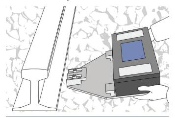
2. Create a small void in the ballast between sleepers and slide the Void Monitor under the rail.
