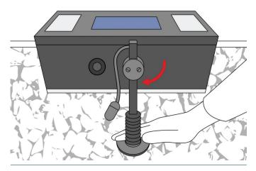
7. Place sensor into the slot on the unit, push in and turn clockwise. The sensor should now stand vertical with the foot resting firmly on the ballast below.
