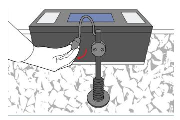
8. Insert the sensor plug and twist it clockwise to establish connection.
