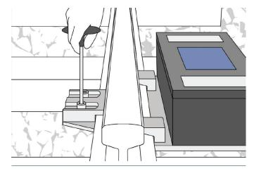
5. Tighten the bolts on the end clamp repeatedly and alternately using the M10 Allen key until secure.
