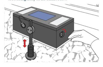
9. Once fitted, check sensor is moving freely with no ballast around it. To turn the unit on, turn on/off switch clockwise so the arrow points to '1'.
