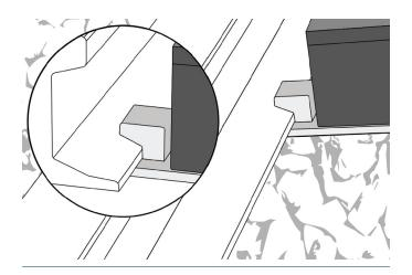
3. Ensure the Void Monitor base plate is flush under the rail. The shoulder should sit on the foot of the rail as shown.
